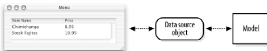
Figure 9-3. A data source as a controller between a model and a view
